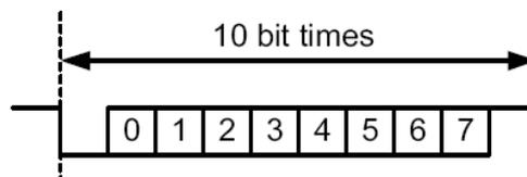
**Figure 2.2:** Byte structure
