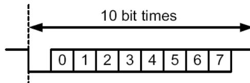
**Figure 2.2:** Byte structure
