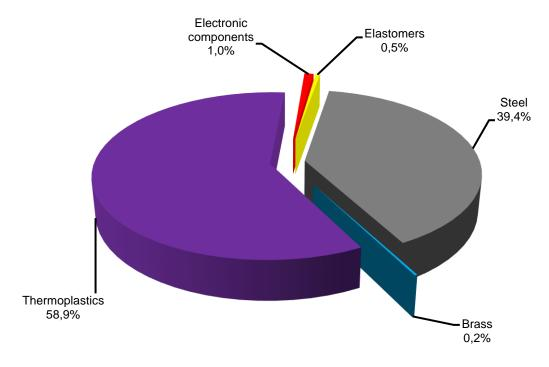
The materials used in the product range and the corresponding weight are disposed below, in *table 1*. The information about the constituent materials is referring to model EB08P-IP65.
