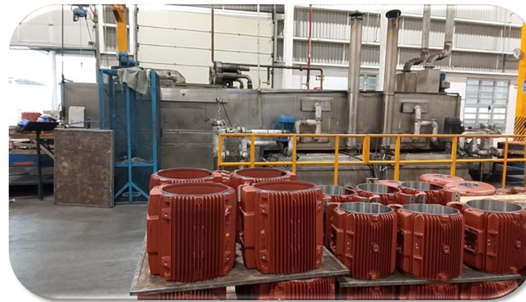
Side view of the component washer, with motor frames in front
