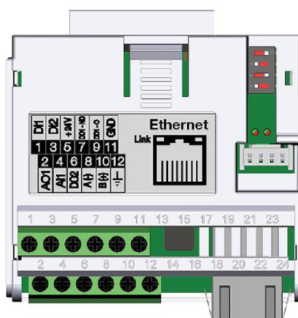
*Figura 20.5: Módulo Plug-in CFW500-CEMB-TCP / CFW500-CETH-IP / CFW500-CEPN-IO*
