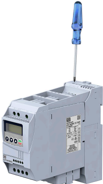
(c) Tighten the screws of the filter set (Torque: 0.51 N/m) (c) Apriete los tornillos del conjunto filtro (Torque: 0.51 N/m) (c) Aperte os parafusos do conjunto filtro (Torque: 0.51 N/m)
