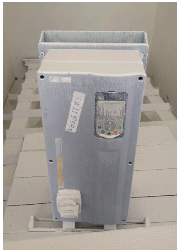
Test with calibrator and dust chamber
