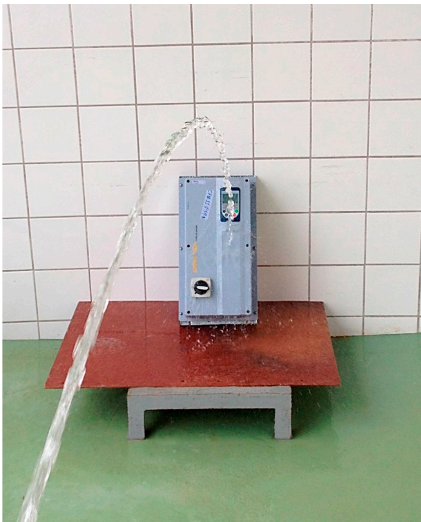
Tests with water jet
