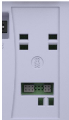
Figure 9 - XC3 bluetooth or ethernet accessory connector.
