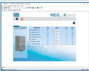
The configuration of the drive is organized in various contextual menus, where the operator through a graphical layout is guided step by step in the configuration process.
