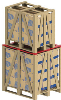
Figure 5.5 – Use of additional battens for stacking
