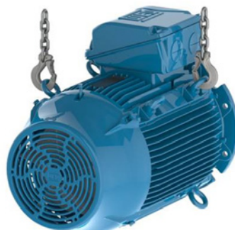
Figure 4.13 – Final result: motor placed in the horizontal position
