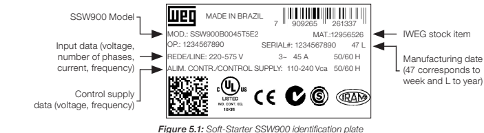
Figure 5.1: Soft-Starter SSW900 identification plate
