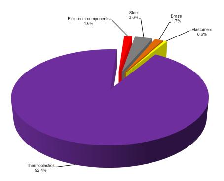
The materials used in the product range and the corresponding weight are disposed below, in *table 1*. The information about the constituent materials is referring to model EB06AP-IP65.
