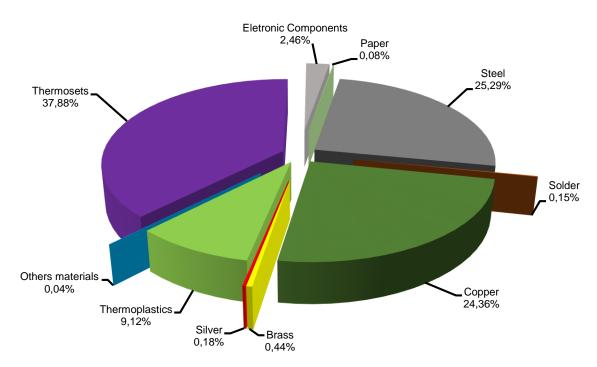
The materials used in the product range and the corresponding weight are disposed below, in *table 1*. The information about the constituent materials is referring to model DWB10000S1000-3ET.
