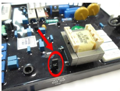
Figure 16.1: Jumper of frequency
