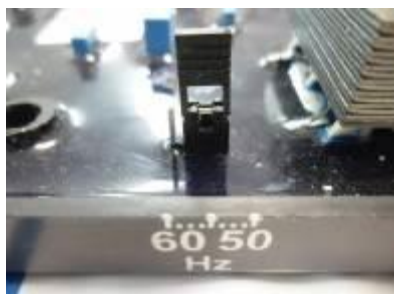
Figure 16.2: Jumper in 50 Hz
