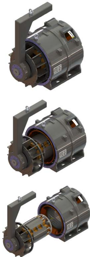
Figure 10.6: Removal of the main rotor with the pendulum device
