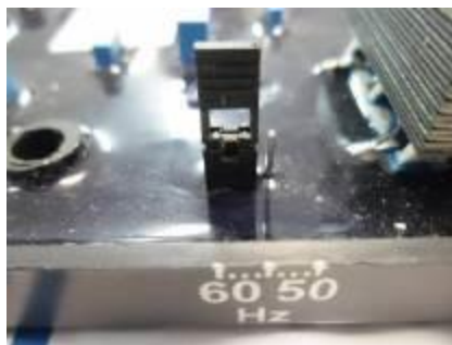
Figure 16.3: Jumper in 60 Hz
