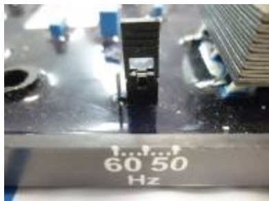
Figure 16.2: Jumper in 50 Hz
