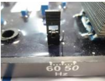
Figure 16.3: Jumper in 60 Hz
