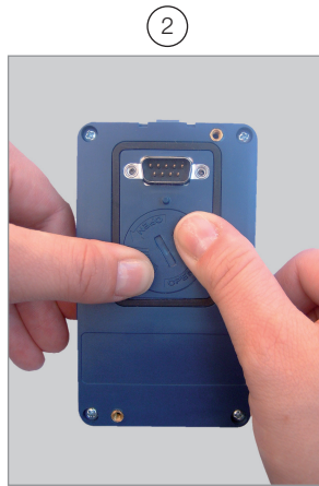
2 Press the cover and rotate it counterclockwise
