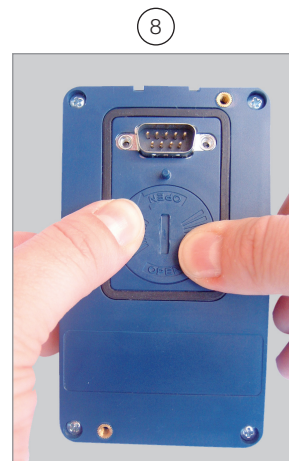
8 Put the cover back and rotate it clockwise
