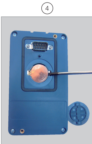
4 Remove the battery with the help of a screwdriver positioned in the right side
