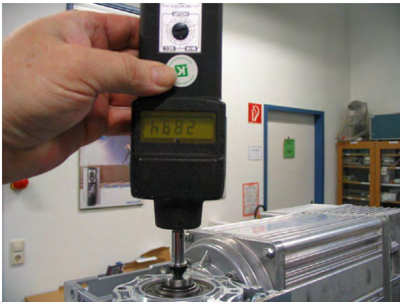
Figure 62: Speed measurement at gear mechanism
