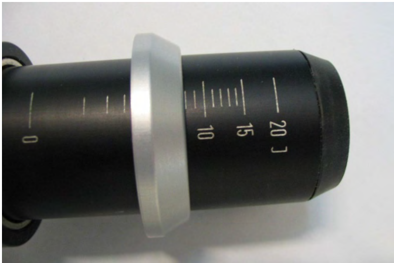
Figure 66: Energy measurement: 8 Joule
