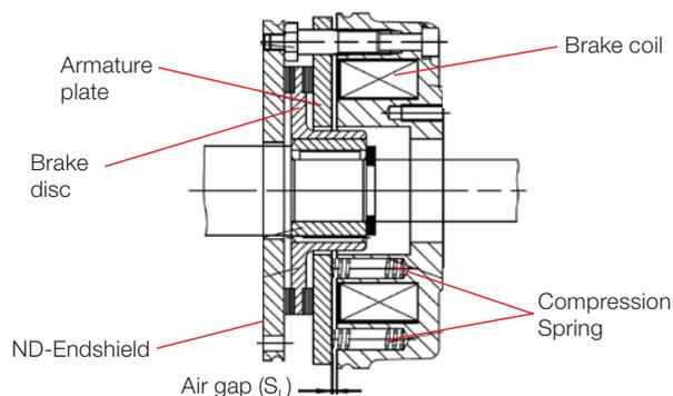
Figure 1 - Scheme of the brake components.
