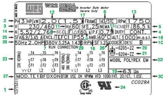
Figure 7 – Nameplate layout for frames 143T to 215T
