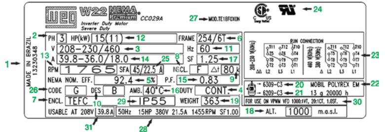
Figure 8 – Nameplate layout for frames 254T to 588/9T
