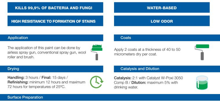
Before starting the painting, all the masonry or concrete must be cured and dry, without fissures, cracks, alveoli and perfectly adhered to the base or other layers of mortar and coating.
