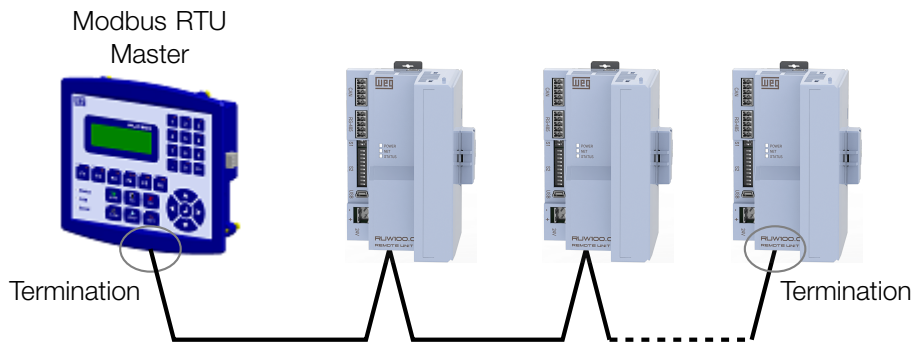
Figure 4.1: Modbus RTU network installation example
