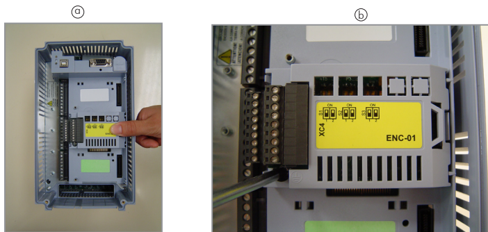
Figure 3: Installation of optional module into slot
