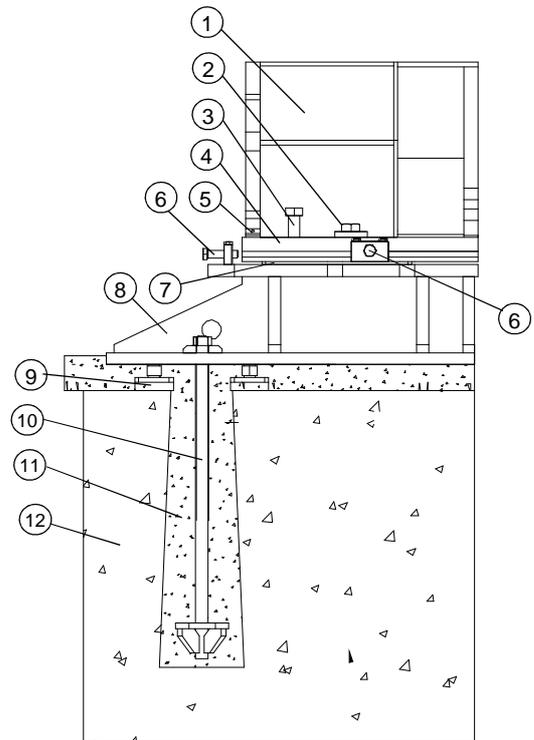
Figure 5.1: Example of anchor base installation
