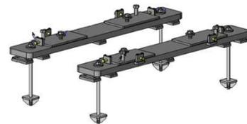
Figure 3.4: Example of soleplate
