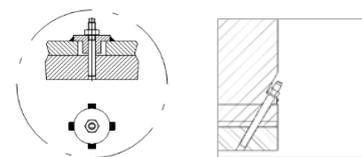
Figure 6.2: Examples of doweling
