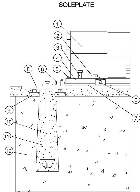
Figure 5.3: Example of soleplate installation
