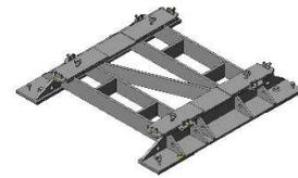
Figure 3.3: Example of intermediate base
