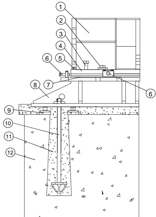
Figure 5.1: Example of anchor base installation
