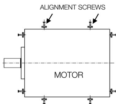
Figure 6.1: Motor horizontal alignment
