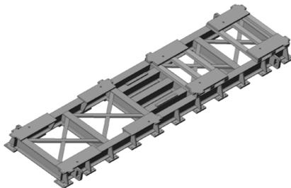
Figure 3.2: Example of common metal base
