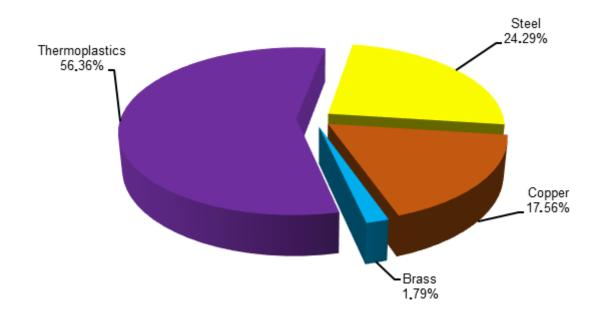
The materials used in the product range and the corresponding weight are disposed below, in *table 1*. The information about the constituent materials is referring to model MSWR 160 B3 H.
