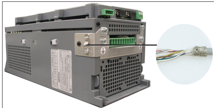
Figure 7.2.4: Connection of shielding (recommended)
