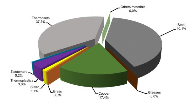
The materials used in the product range and the corresponding weight are disposed below, in *table 1*. The information about the constituent materials is referring to model CWM250-22-30D24.
