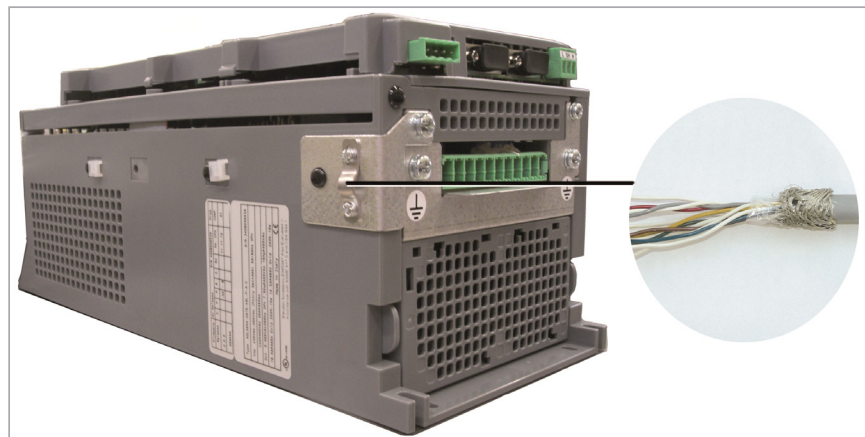
Figure 7.2.5: Connection of shielding (recommended)
