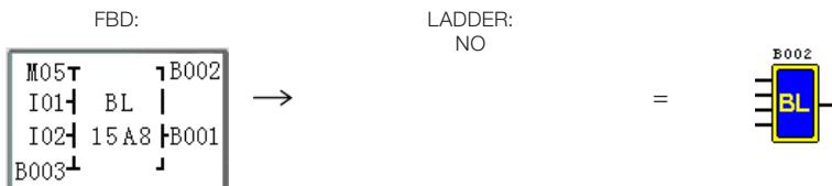
**Note:** When an input terminal is connectionless (NOP), it will be considered in low level (Lo).
