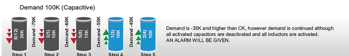
Figure 3.28: PFW03-T des. Sequential mode
