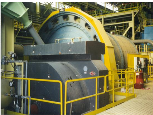
Metso Minerals – Minera Alumbrera – Argentina Ball Mill – 8000HP, 34 Poles, 3PH / 50 Hz / 6.6 kV
