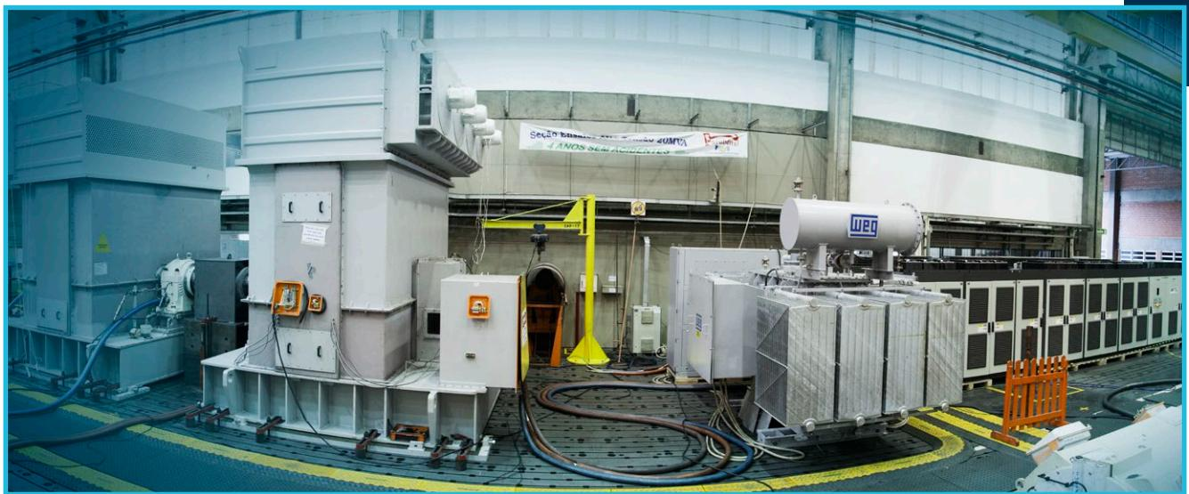
*Combined test (MV Incoming Switchgear + Phase-shifting Transformer + MV VSD + MV Motor)*
