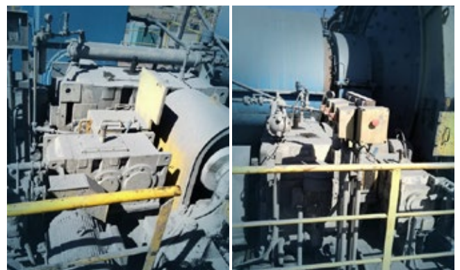
NX Gold - Nova Xavantina - Brazil Single pinion ball mills: Slip ring motor + Main gearbox + Flexible couplings + Squirrel cage motor + Auxiliary gearbox
