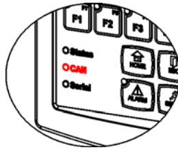
Figure 2.2: Indication LED of CAN interface
