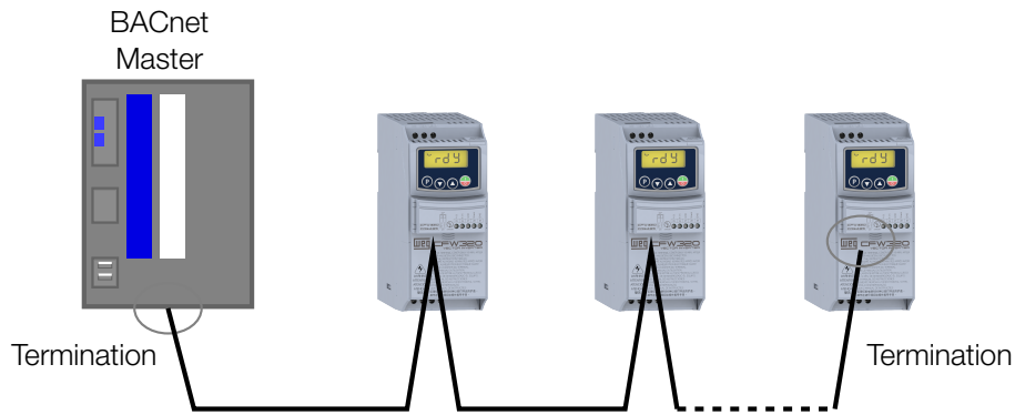
Figure 4.1: BACnet network installation example
