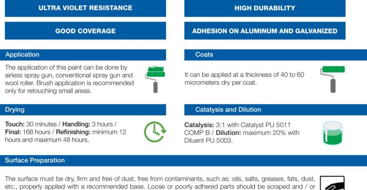
brushed. On aged paint, sand superficially, leaving the surface free of brightness and remove loose particles. In walls with new plaster, it is recommended to use the Epoxy W-POXI CVS 301 sealer.
