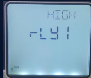
Relay is triggered when the upper limit is reached
