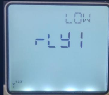
Relay is triggered when the lower limit is reached
