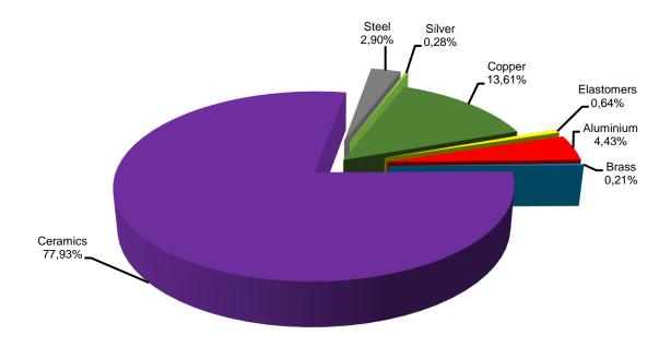
The materials used in the product range and the corresponding weight are disposed below, in *table 1*. The information about the constituent materials is referring to model NH aR FNH00-80K-A
