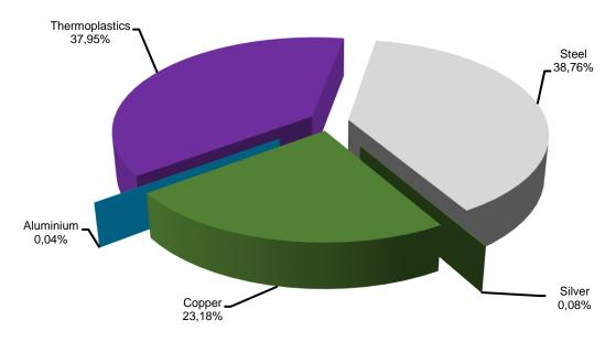
The materials used in the product range and the corresponding weight are disposed below, in *table 1*. The information about the constituent materials is referring to model MDW (70 -125A) 1P.
