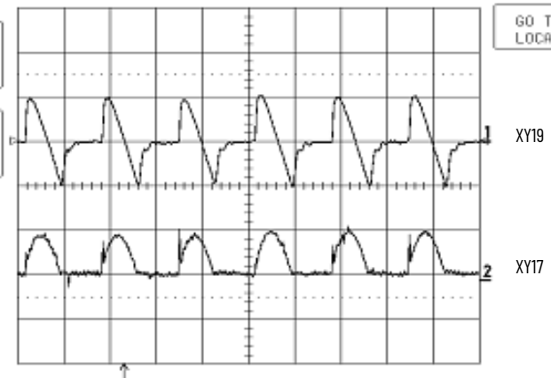
Figure 7 - Good SCR Armature Voltage and Motor Current Signal Example
