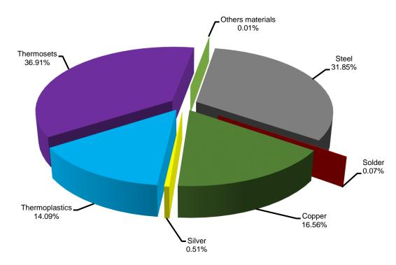
The materials used in the product range and the corresponding weight are disposed below, in *table 1*. The information about the constituent materials is referring to model DWB160N160-4DFT.
