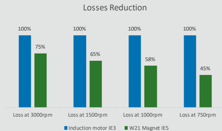
Figure: Comparison between Cast Iron IE3, W21 Magnet GB1 - 315kW - 3000 RPM
