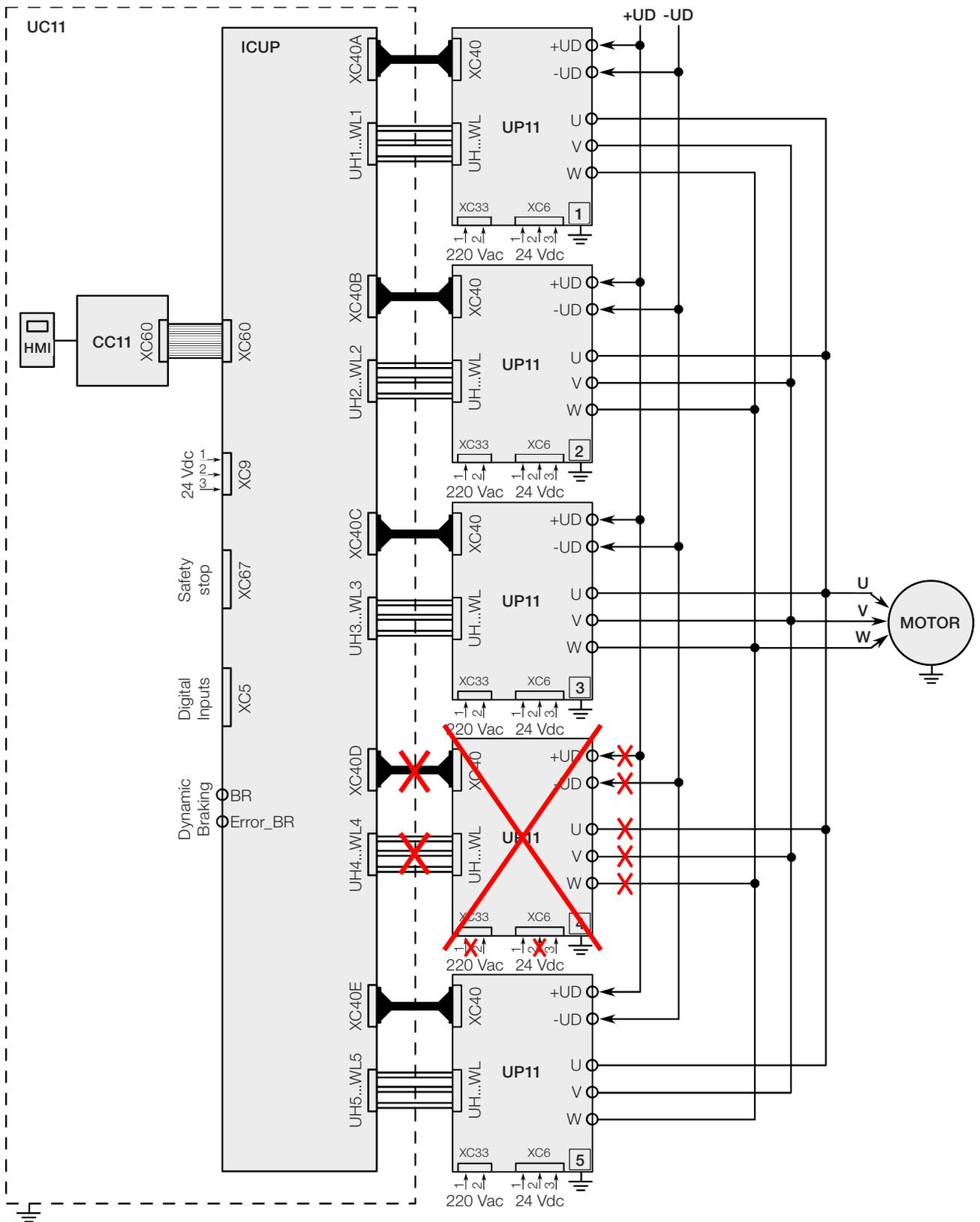
Figure 5.6: Disconnection of the power and control cables of UP11 number 4
