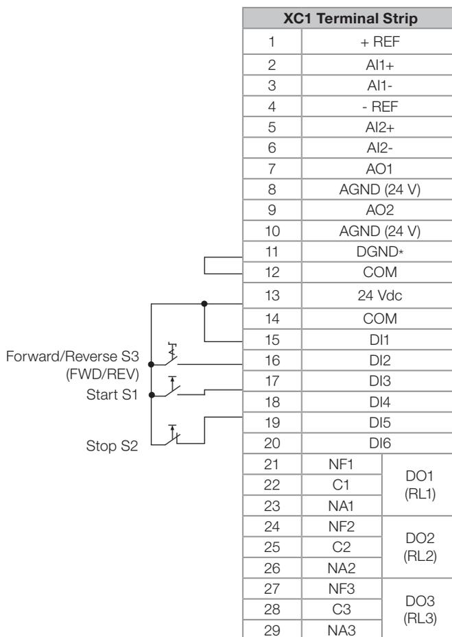
Figure 3.45: XC1 wiring for control connection # 3
