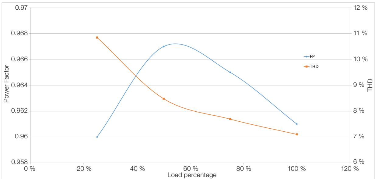
**Figure 3.19:** Power Factor (FP) and THD (I) with variation of the output power. 12-pulse rectifier
