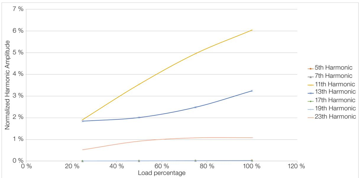
**Note:** Amplitude of the normalized harmonics as a function of the fundamental with 100 % of load. 12-pulse rectifier.
