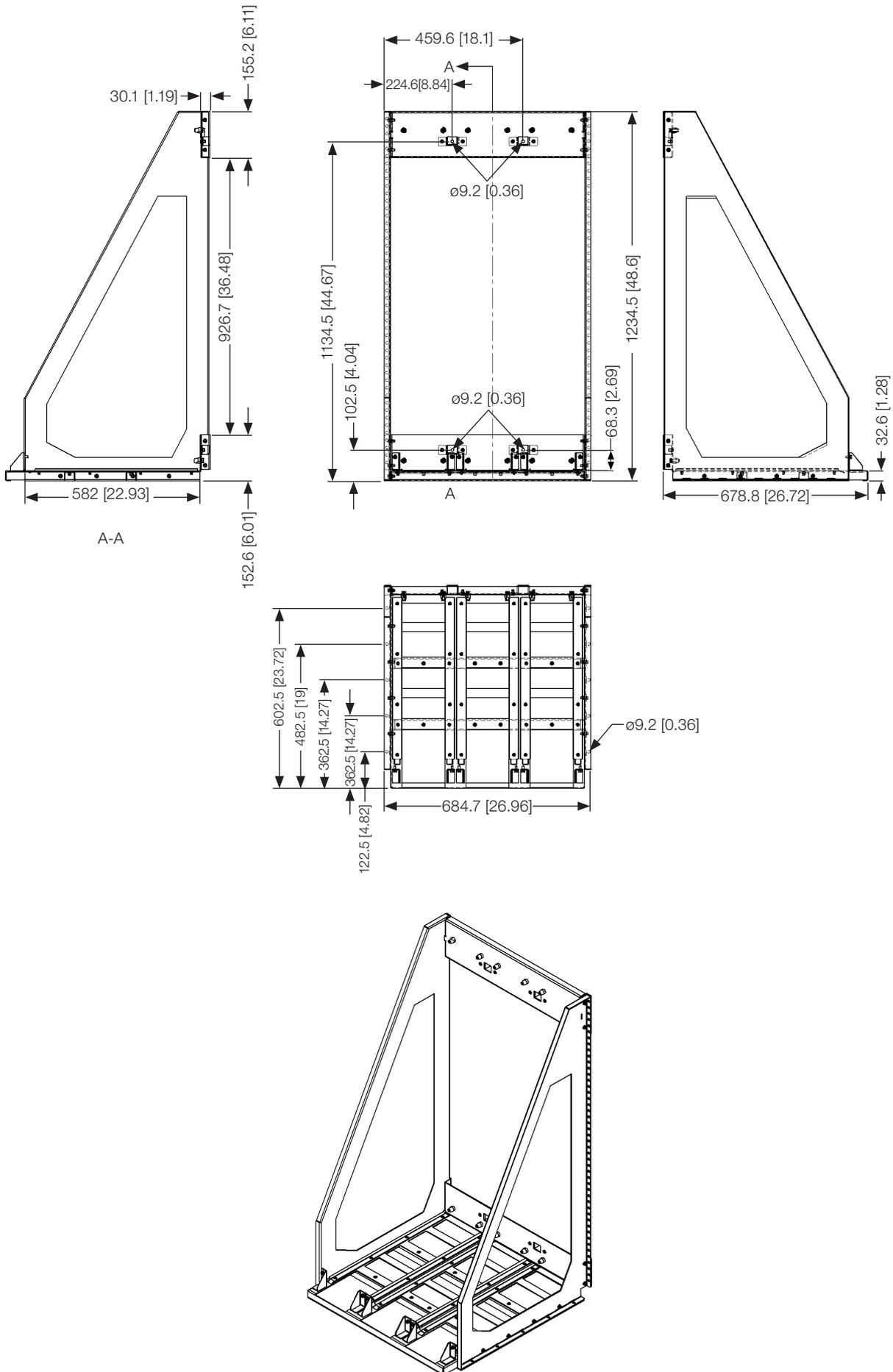
Figure 3.4: Dimensions of Rack 3 G2 in mm [in]
