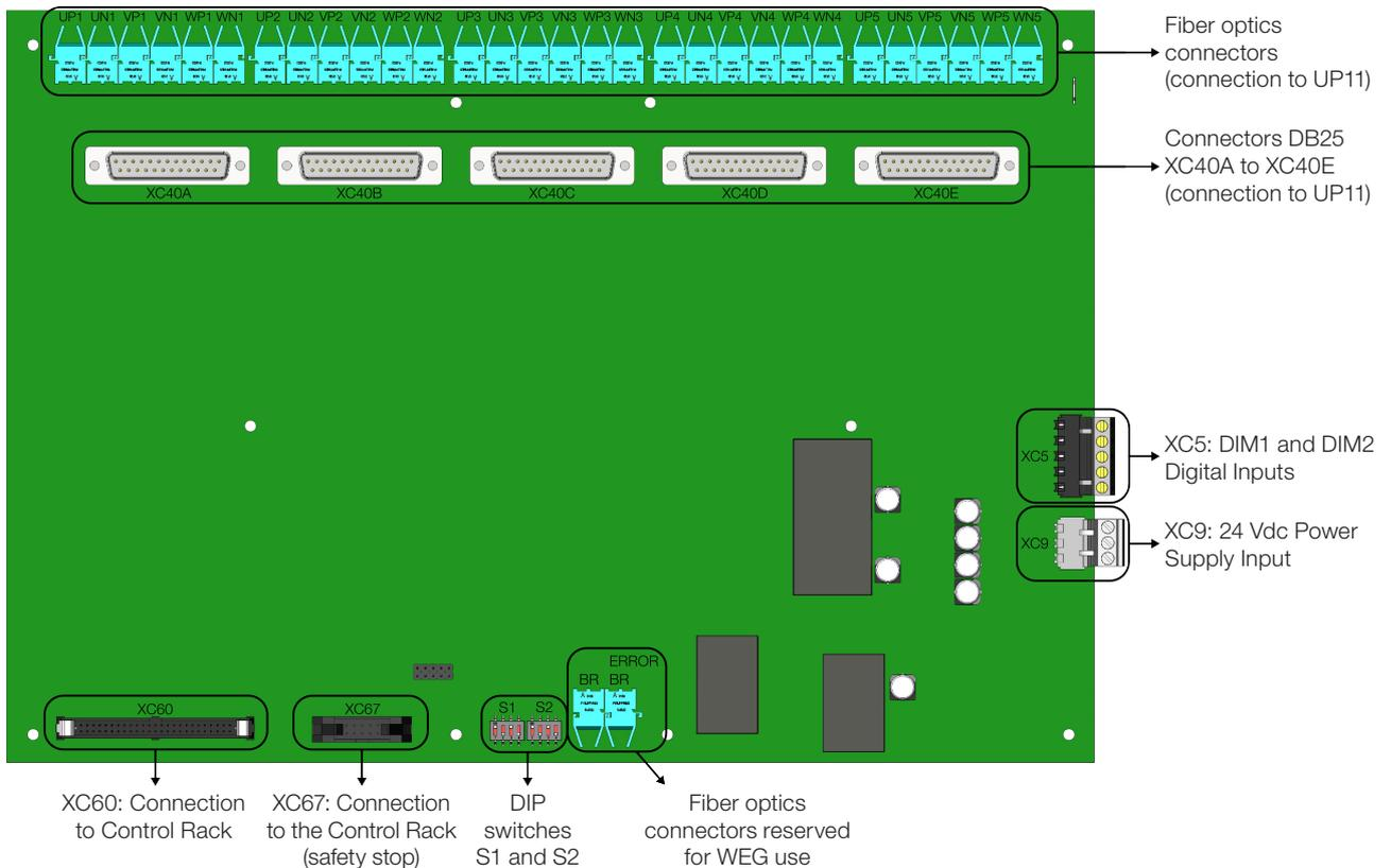
**Figure 3.33:** ICUP board connection points
