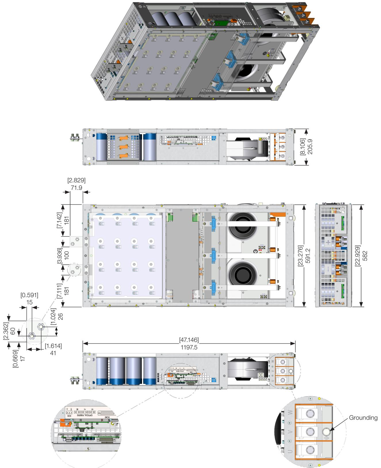
Figure 8.2: Mechanical dimensions in mm [in]
