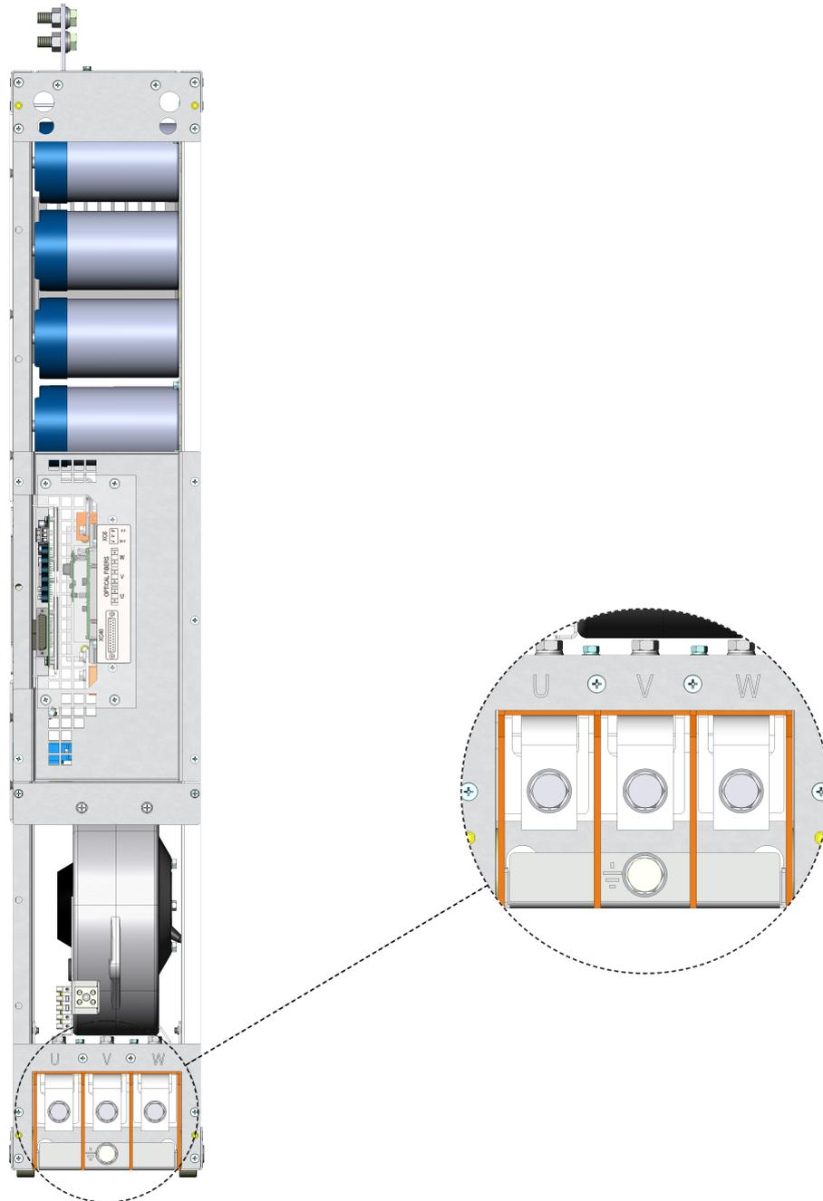
Figure 3.25: U, V, W and grounding terminals
