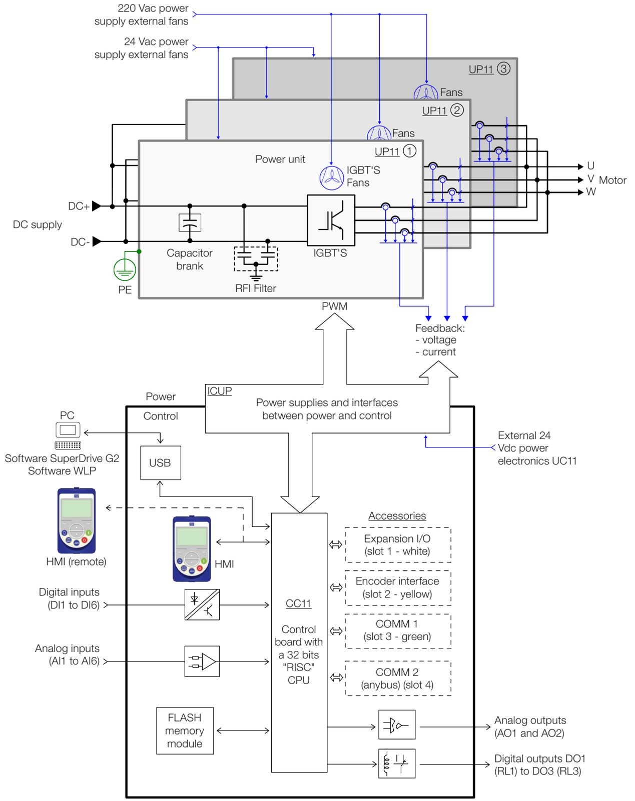
Figure 2.1: Block diagram for the CFW-11M G2
