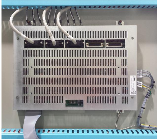
Figure 3.36: ICUP shield fastened to the panel
