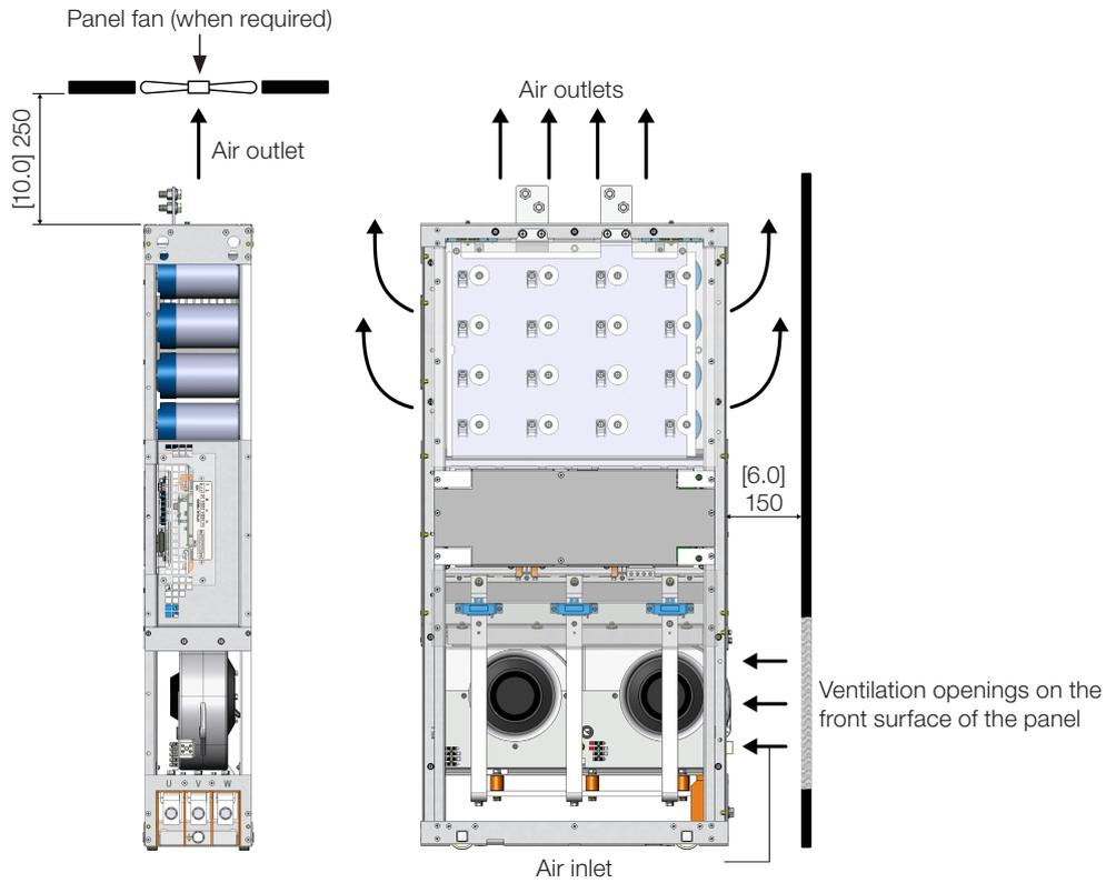
Figure 3.2: Clearances for ventilation in mm [in]
