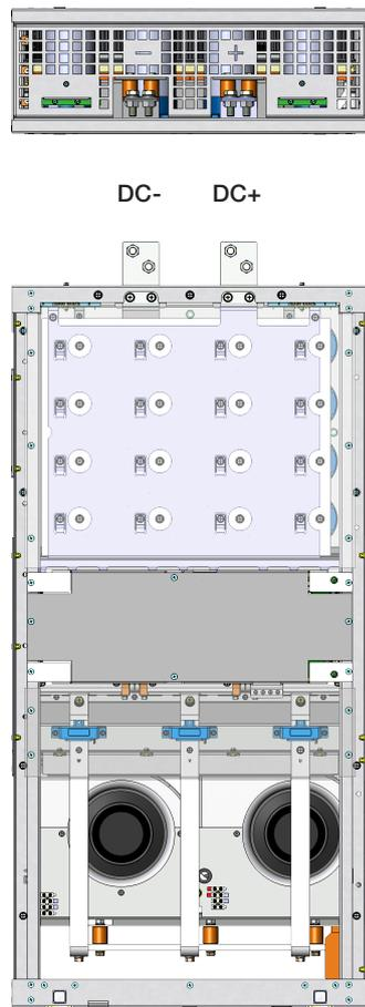
Figure 3.24: DC power supply terminals
