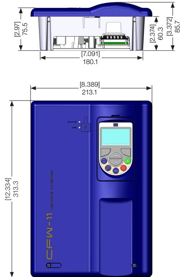
Figure 8.3: Control rack dimensions in mm [in]
