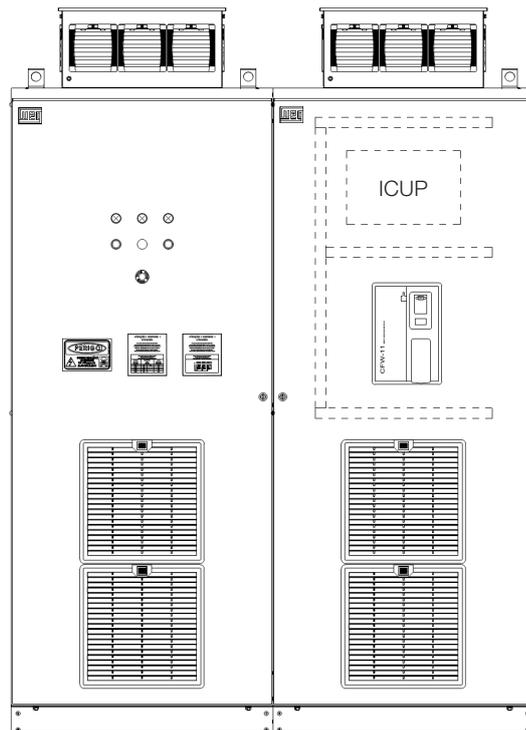
Figure 3.12: Example of mounting of the control rack in the panel
