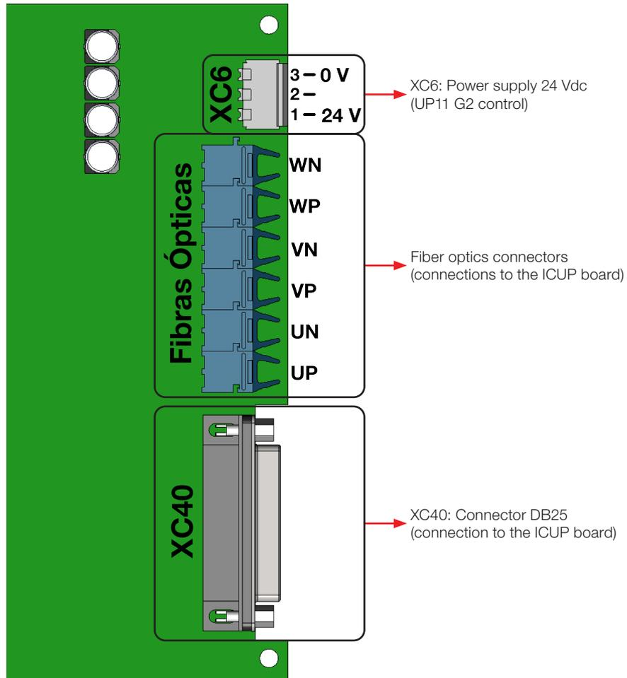
Figure 3.31: Identification of the control connections of the UP11 G2
