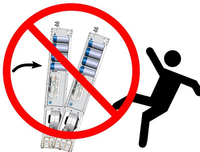
**Figure 2.8:** Do not tilt the power units
