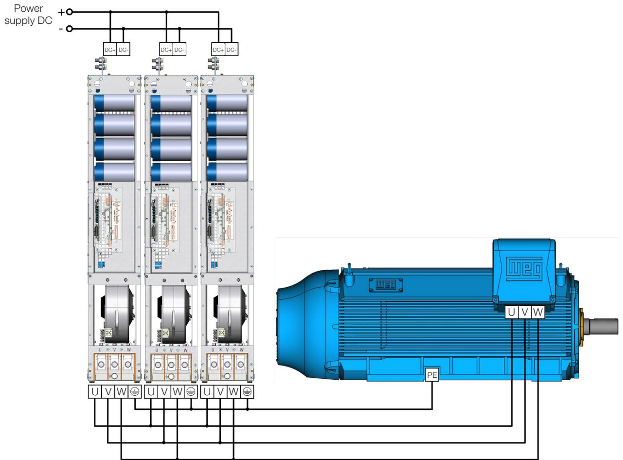
Figure 3.23: Power and grounding connections
