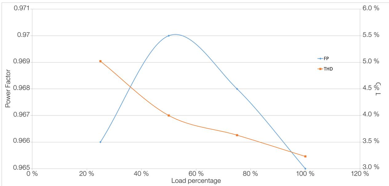
**Figure 3.21:** Power Factor (FP) and THD (I) with variation of the output power 18-pulse rectifier
