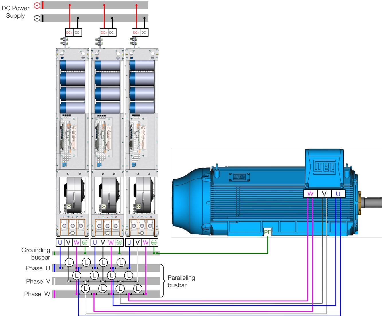
Figure 3.26: Recommended distribution for the motor cables
