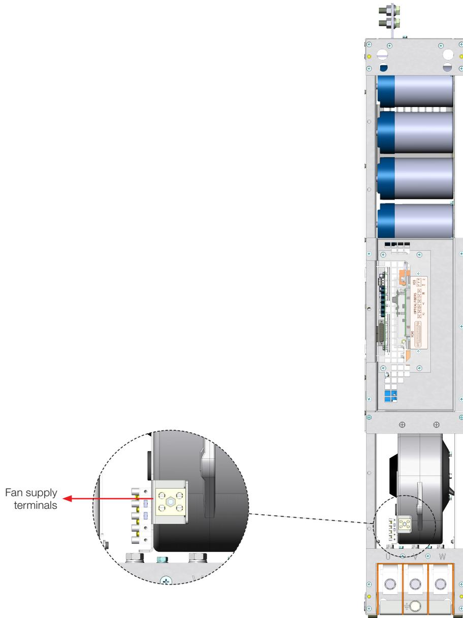
Figure 3.32: Fan supply terminals
