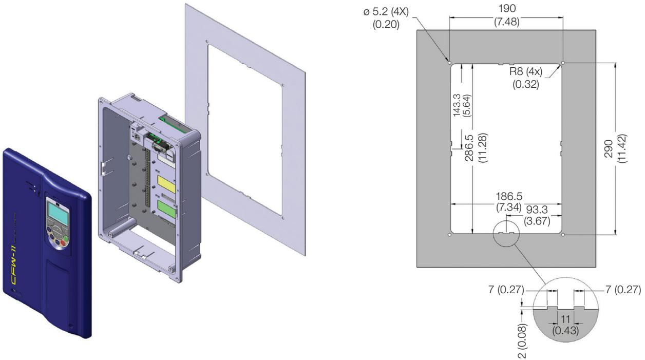
Figure 3.13: Mounting of the control rack and necessary slots mm (in)
