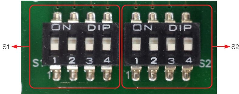
Figure 3.34: DIP switches S1 and S2 detail
