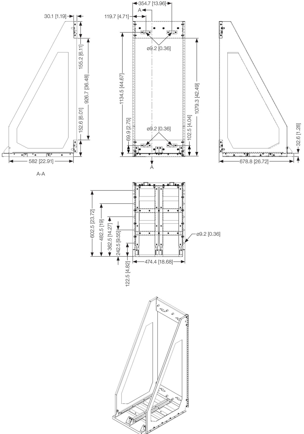
Figure 3.3: Dimensions of Rack 2 G2 in mm [in]
