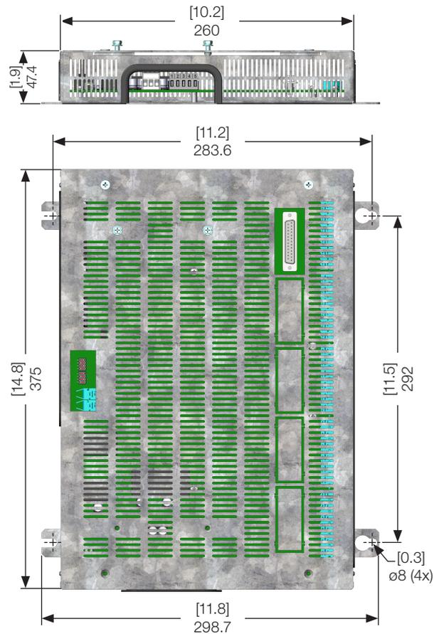
Figure 8.4: Dimensions of the ICUP board metal enclosure in mm [in]
