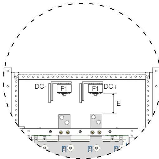
**Figure 3.27:** Side view of the connections of the flexible braids and fuses
