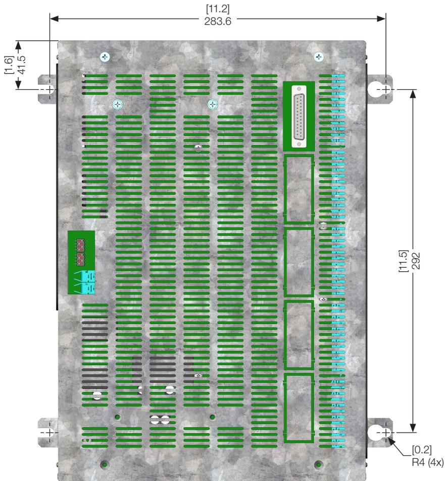
Figure 3.14: Mounting of the base of the ICUP1 module (mm)
