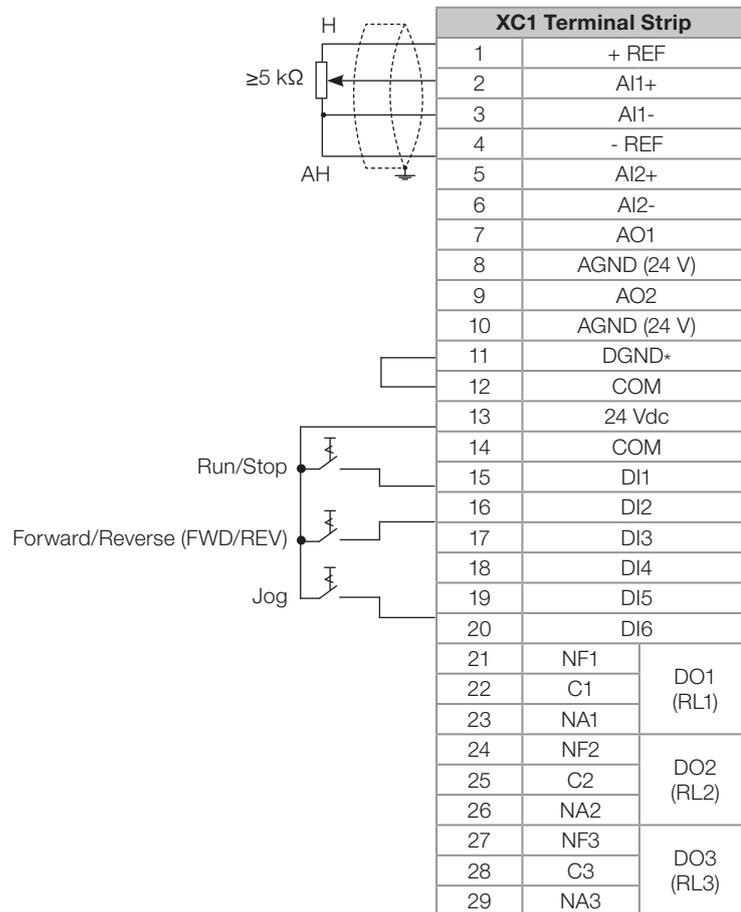
**Figure 3.44:** XC1 wiring for Control Connection #2
