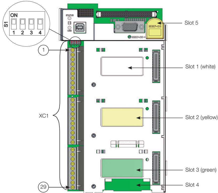
**Figure 3.41:** Connector XC1 and switches to select the signal type of the analog inputs and outputs
