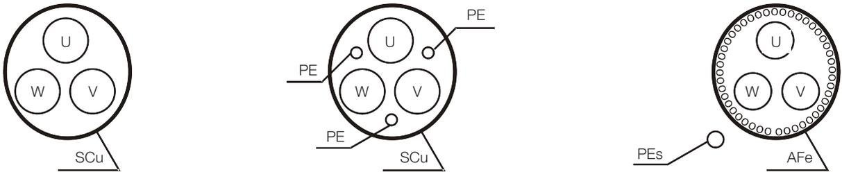
Symmetrical shielded cables: three concentric conductors with or without a ground conductor, symmetrically manufactured, with an external shield of copper or aluminum.
