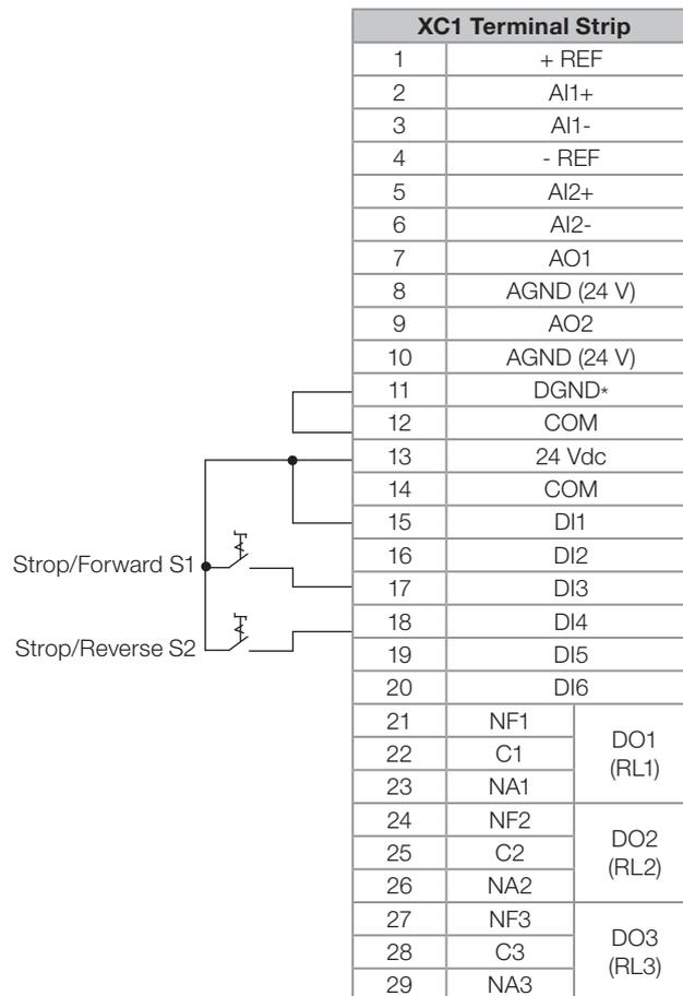
**Figure 3.46:** XC1 wiring for control connection # 4
