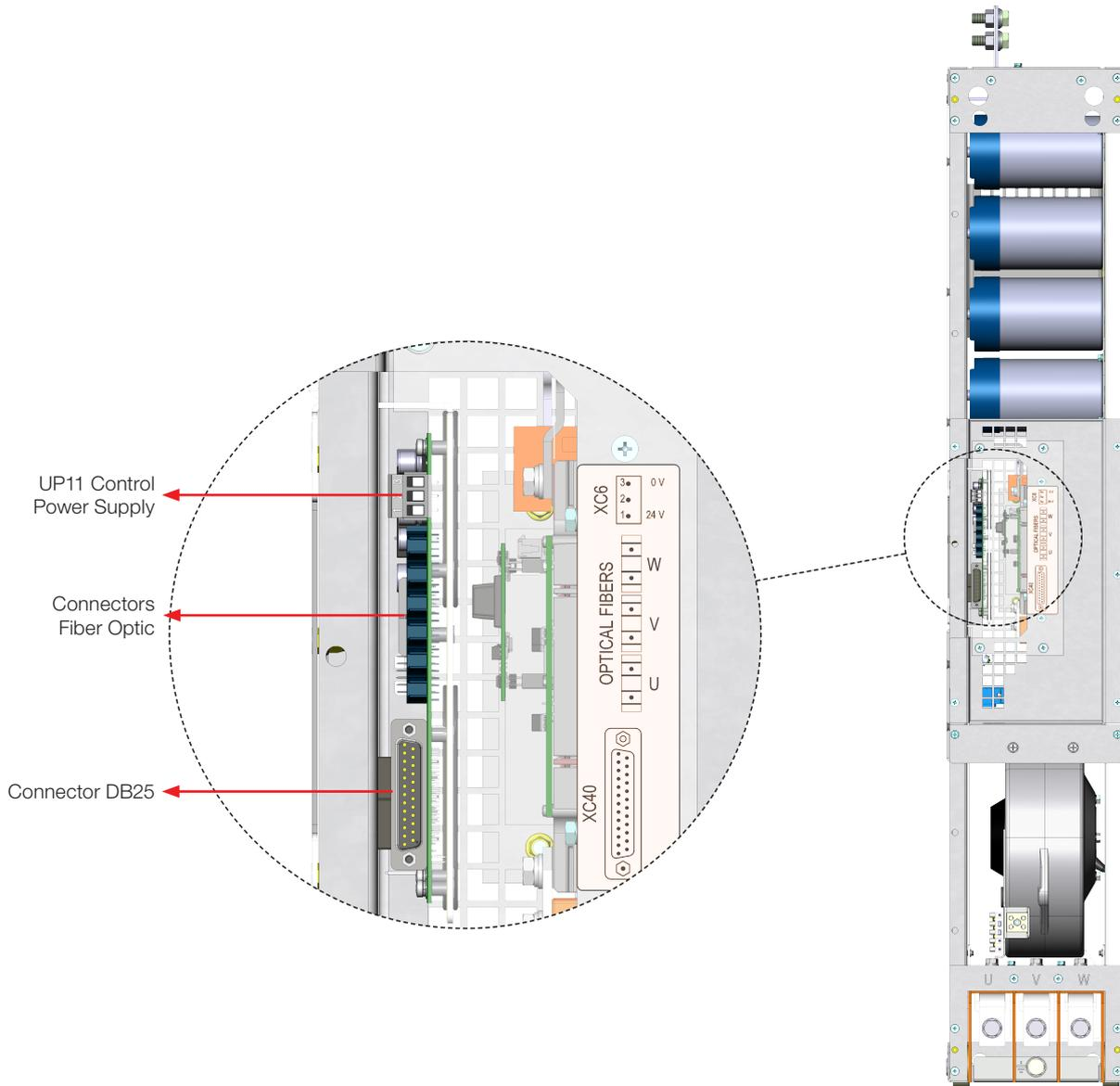
Figure 3.30: Control cable connection points on the UP11 G2
