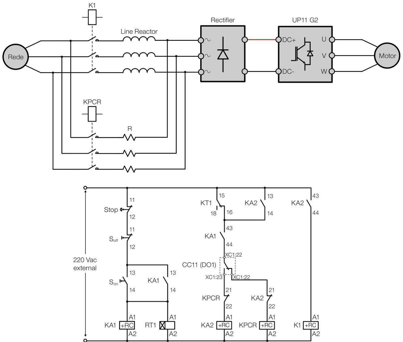
Figure 3.15: Pre-charge circuit example
