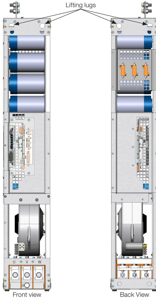
Figure 3.1: UP11 G2 lifting lugs
