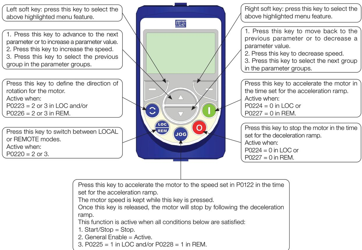
Figure 4.1: HMI Keys
