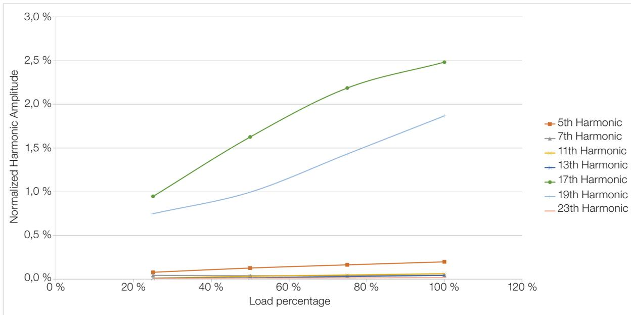
**Note:** Amplitude of the normalized harmonics as a function of the fundamental with 100 % of load. 18-pulse rectifier.
