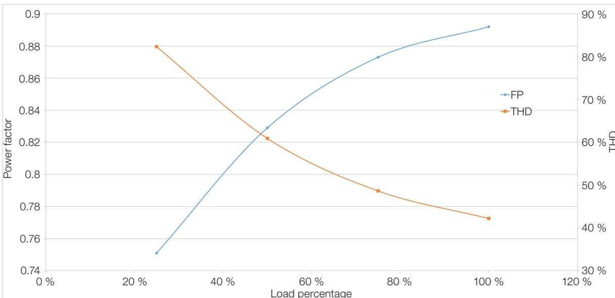
**Figure 3.17:** Power Factor (FP) and THD(I) with variation of the output power 6-pulse rectifier
