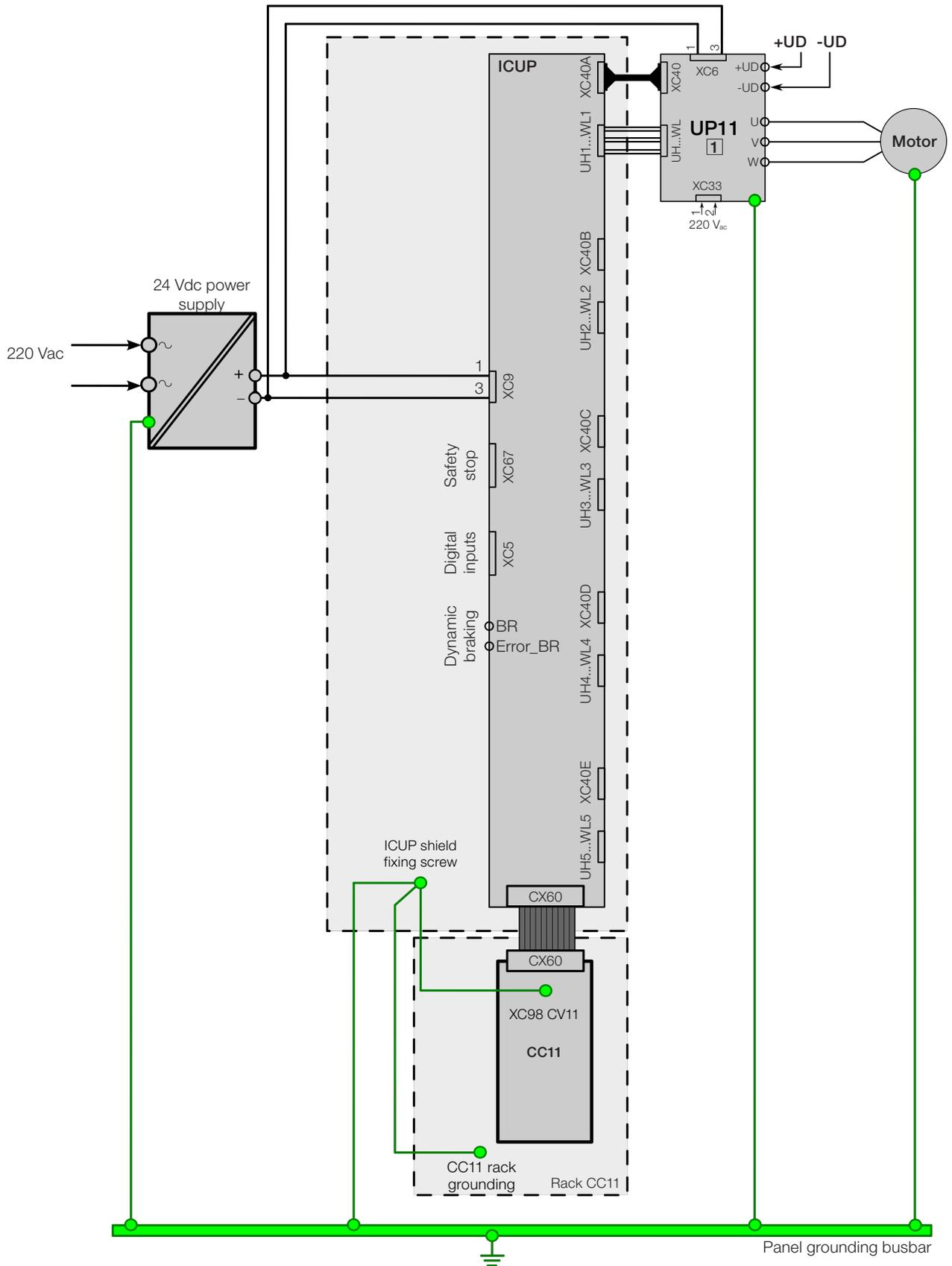
Figure 3.35: Grounding diagram of the UP11 plus UC11, in case of only one UP11
