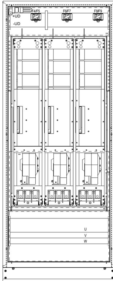
Figure 3.11: Column with 3 UP11 G2 installed
