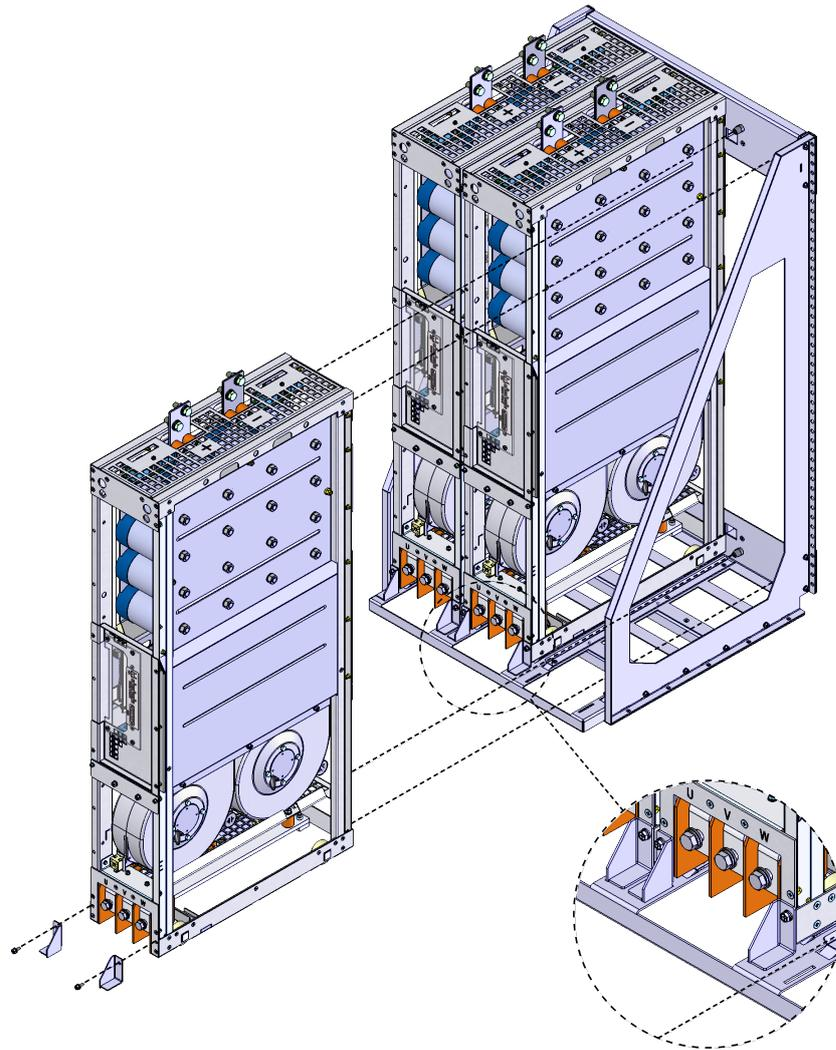
Figure 3.5: Insertion of the power modules into Rack 3 G2
