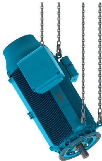
Figure 4.16: Placing HGF, W50 and W51 HD motors in vertical position
