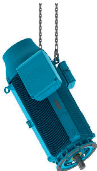
Figure 4.17: Lifting HGF, W50 and W51 HD motors by the eyebolts at the non-drive end
