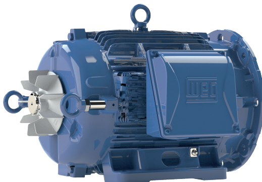
Figure 4.14: Eyebolts with extension fixed at NDE side to place the motor in vertical position, with the shaft end down (V5/V35)
