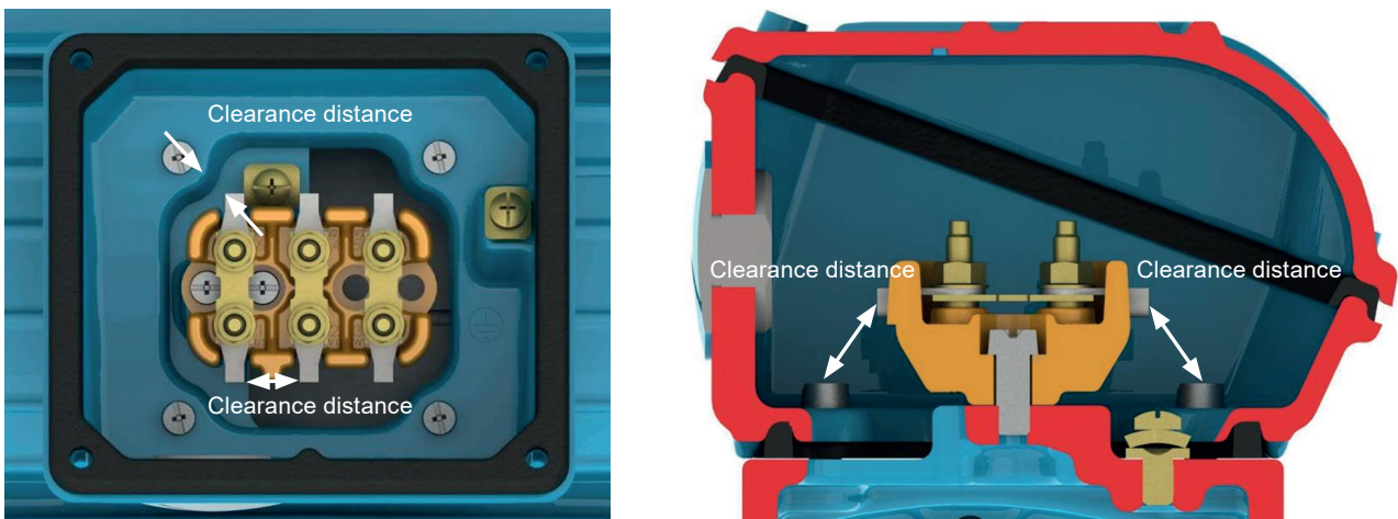
Figure 6.16: Minimum clearance distance (mm) x supply voltage
