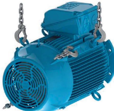
Figure 4.11: Installation of the second pair of eyebolts
