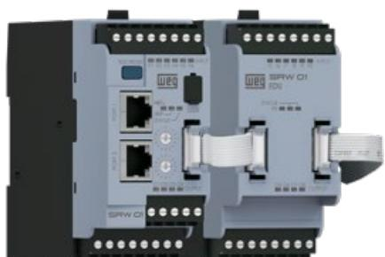
The Digital Expansion Unit (EDU) increases the number of digital inputs and outputs present in the Control Unit (UC) of the SRW01. The EDU adds 6 digital inputs and 4 digital outputs, and can be used to monitor signals and to control external devices.
