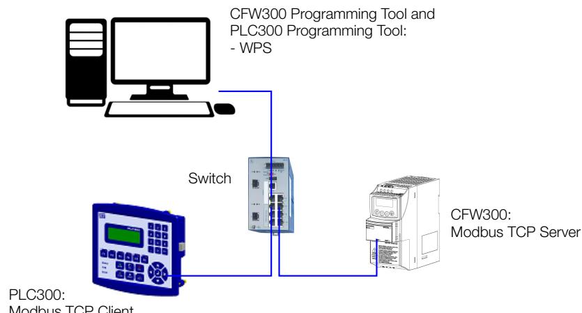
Figure 1.1: Network components for this application
