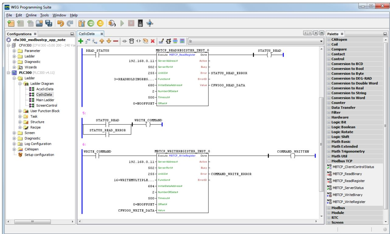
Figure 4.3: Ladder Logic to Read/Write Server Data
