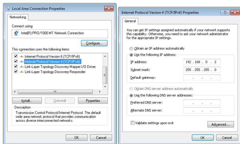
Figure 2.1: PC IP Address Configuration
