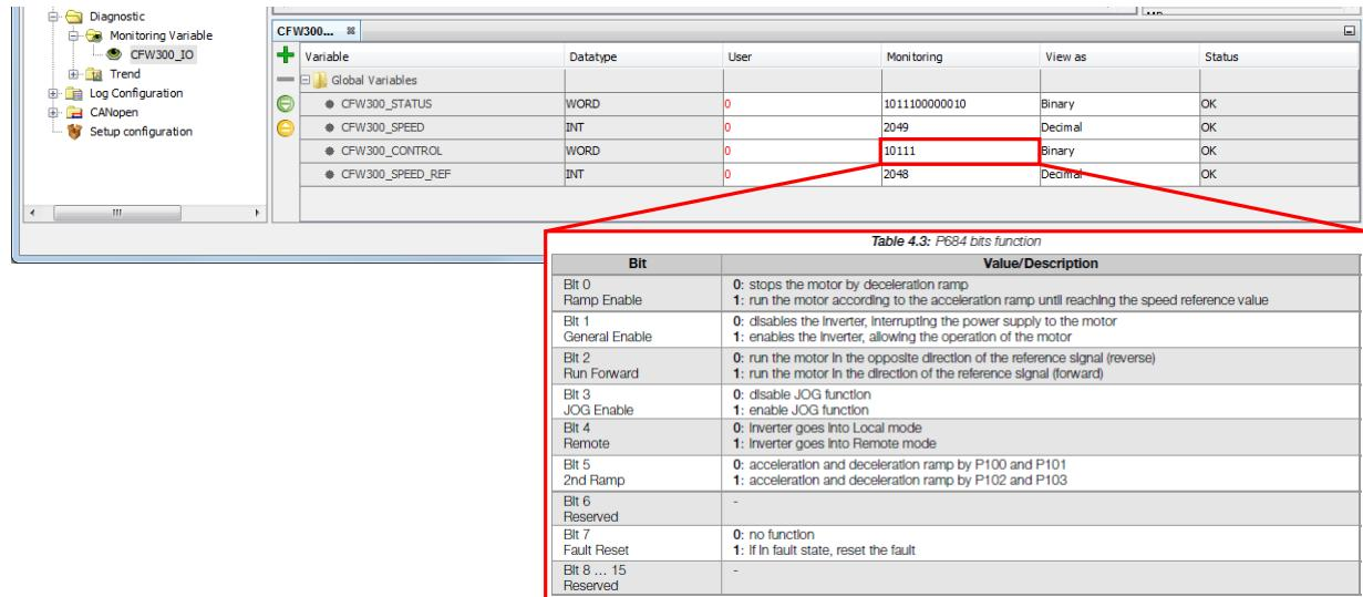
**Figure 5.3:** Write data, with highlight to the command word as described at CFW300 Modbus TCP documentation
