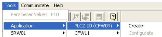
In this example, by clicking on the “create” option, an application for the PLC 2 will be created, where a
