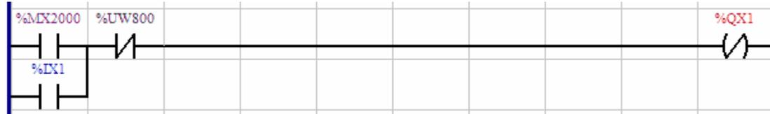
If the bit marker 2000 or the digital input 1 is 1, and the user parameter 800 is 0, write 0 to the digital output 1, otherwise, writes 1.
