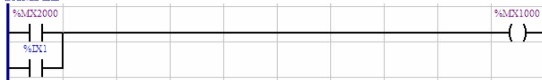
If the bit marker 2000 or the digital input 1 is 1, writes 1 in the bit marker 1000. Otherwise, writes 0.
