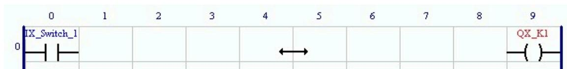
Figure – Position between NO contact and coil.
