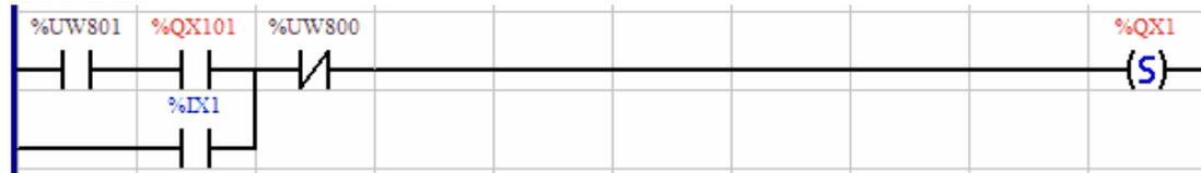
If the user parameter 801 and the digital output 1 of the drive are 1, or the digital input 1 is 1 and the user parameter 800 is 0, it sets the digital output 1. Otherwise, the output value is maintained.
