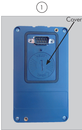
1 Cover for battery access
