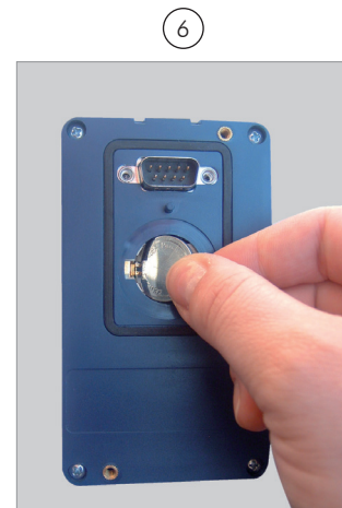
6 Install the new battery positioning it first at the left side
