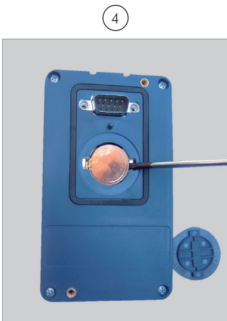
4 Remove the battery with the help of a screwdriver positioned in the right side
