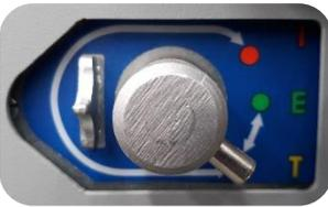
**TESTING Position (T):** Power stabs are disconnected from the busbar and control stabs are connected. In this position it is possible to perform tests on the functional units without voltage in the power terminal block
