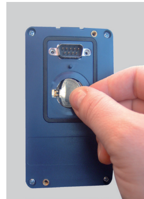
Install the new battery positioning it first at the left side
