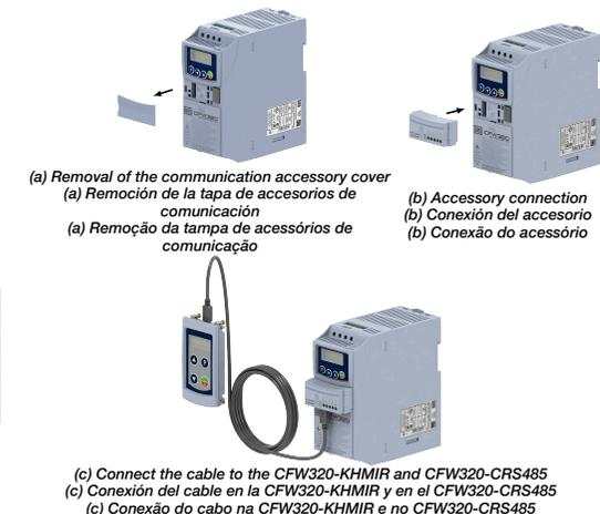
**Figure A.1:** (a) to (c): Installation of accessory
