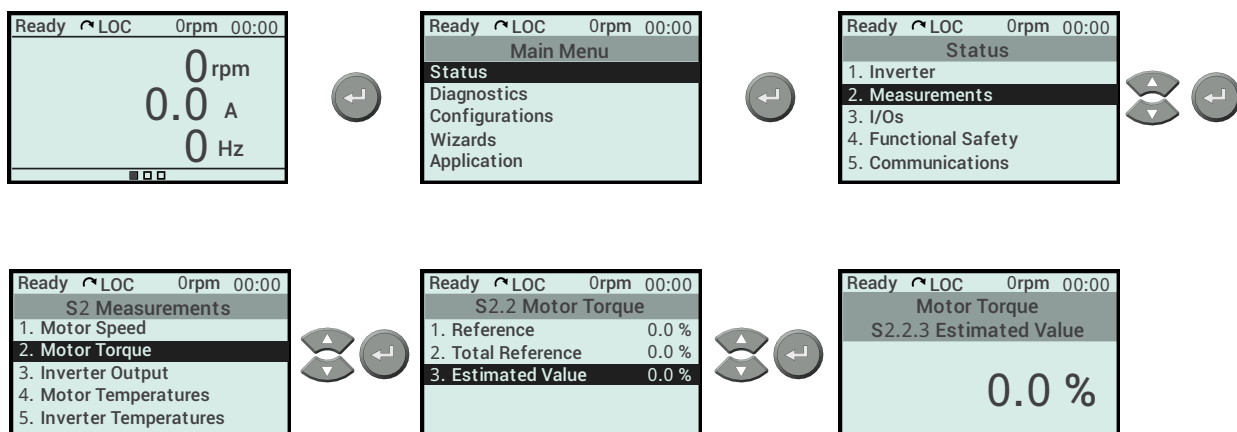
Figure 8.4: Estimated motor torque reading
