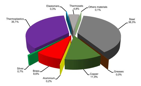
The materials used in the product range and the corresponding weight are disposed below, in *table 1*. The information about the constituent materials is referring to model CWM25-00-30D24.
