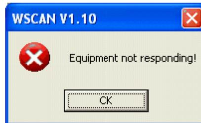
In this case, check the serial cable connection between the serial port on the PC and the board serial connector. Besides that, verify the serial configuration set in the WSCAN software as well as the board configuration.
